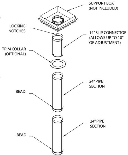
If the ceiling is higher than 8 feet, obtain Pipe Sections from your dealer to accommodate the additional height. Pipe Sections are available in 1', 2' and 4' lengths. (10" diameter pipe available in 1' and 2' lengths only)
